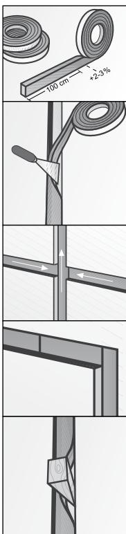
**Preparation of joint/application base:** The substrate/pressure section base should be as level as possible and cleaned (e.g. plaster leftovers removed completely). The joints should run parallel where possible (in some cases a re-plastering or re-profiling of the joints in older buildings could be necessary). The specified joint sealing tape range must not be exceeded or fallen below. This also applies for sections with uneven surfaces.
