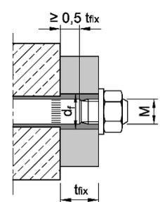
The annular gap in the clearance hole in the fixture has to be filled completely by excess mortar!
