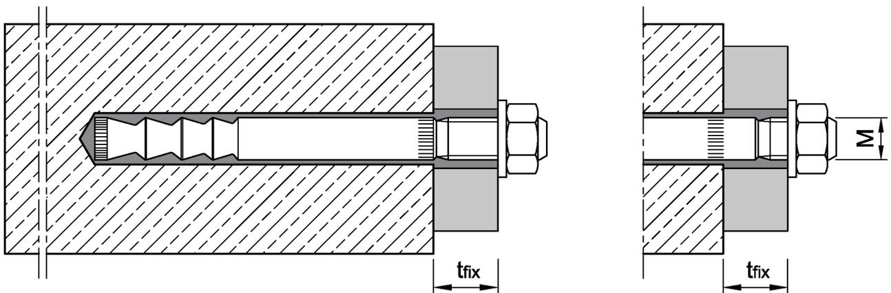
Anchor rod **VMZ-IG** with internal thread<sup>1)</sup>
