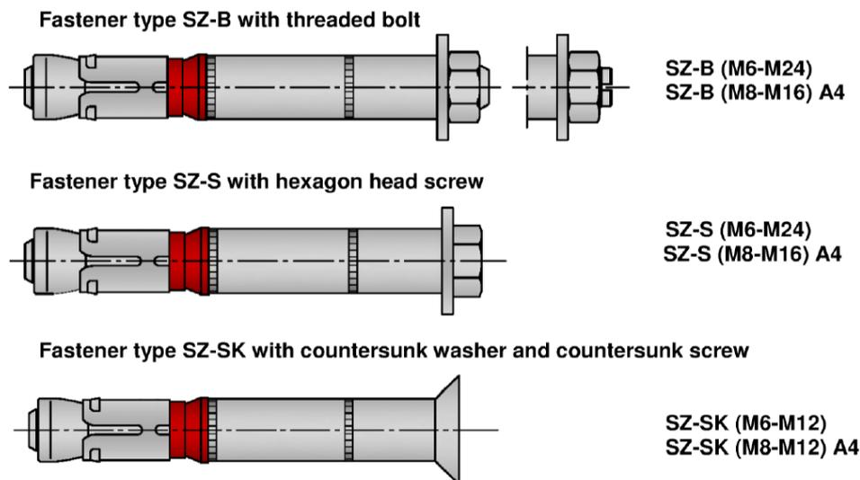
Figure 1-1: Schematic drawing of the anchors SZ for steel fiber reinforced concrete as different types SZ-B, SZ-S and SZ-SK.
