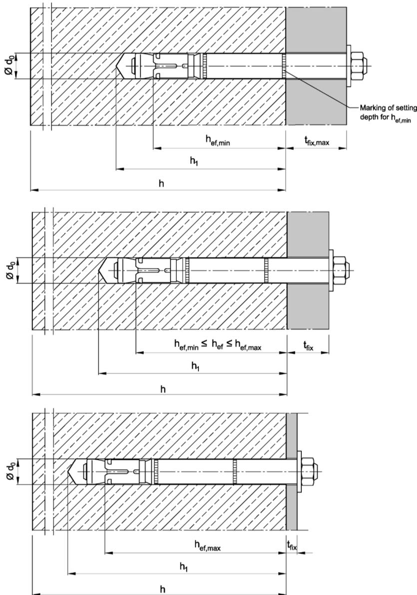
Figure 2-1: Example of an installation situation and nomenclature of the dimension after installation in steel fiber reinforced concrete.
