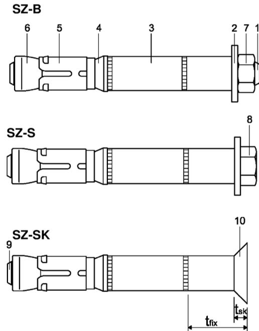
Figure 2-2: Drawing of the MKT anchor system SZ and single parts of an anchor.
