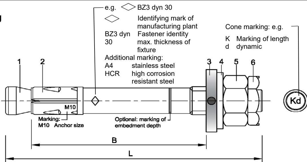
**Usable length:**  $B = h_{\text{ref}} + t_{\text{fix}}$
