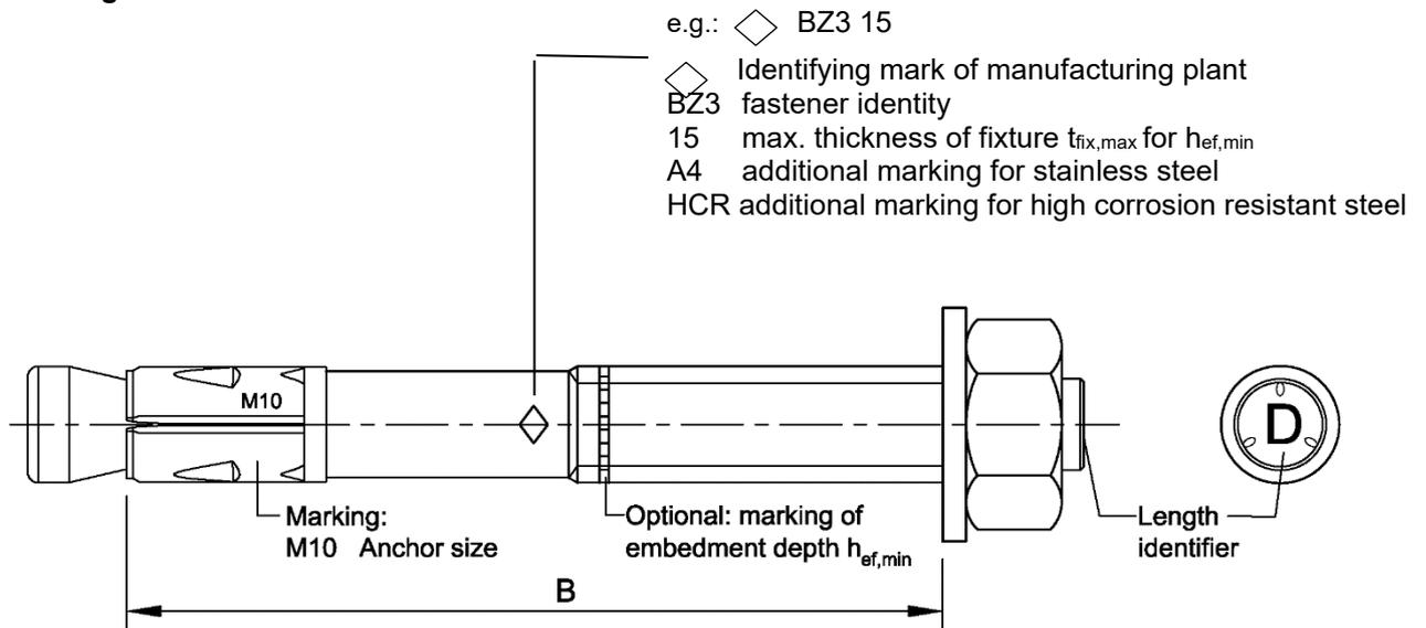
Usable length: **B = h<sub>ef</sub> + t<sub>fix</sub>**
