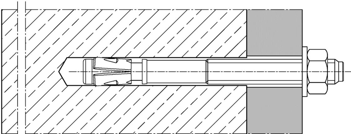
**Installation condition with filling washer (optional with cap nut)**
